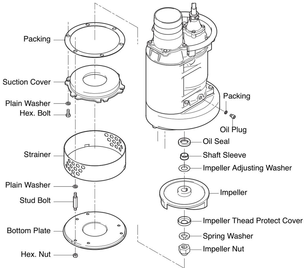
**Note:** *The above exploded view is for model KRS2-C6. Other models may differ slightly in shape and construction.*
