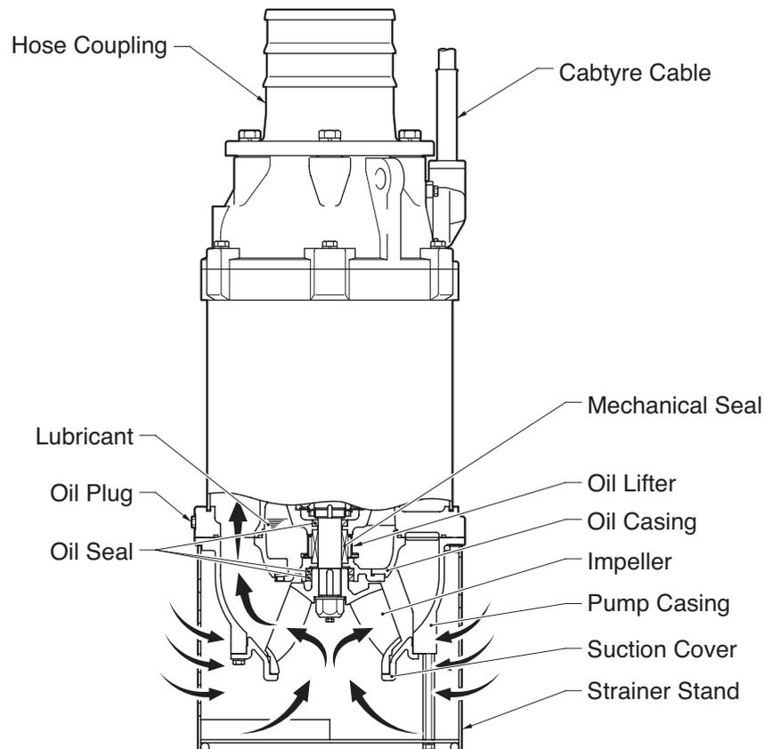
**Note:** *The above diagram is typical of the KRS1022, but some models may vary slightly in appearance or internal structure.*
