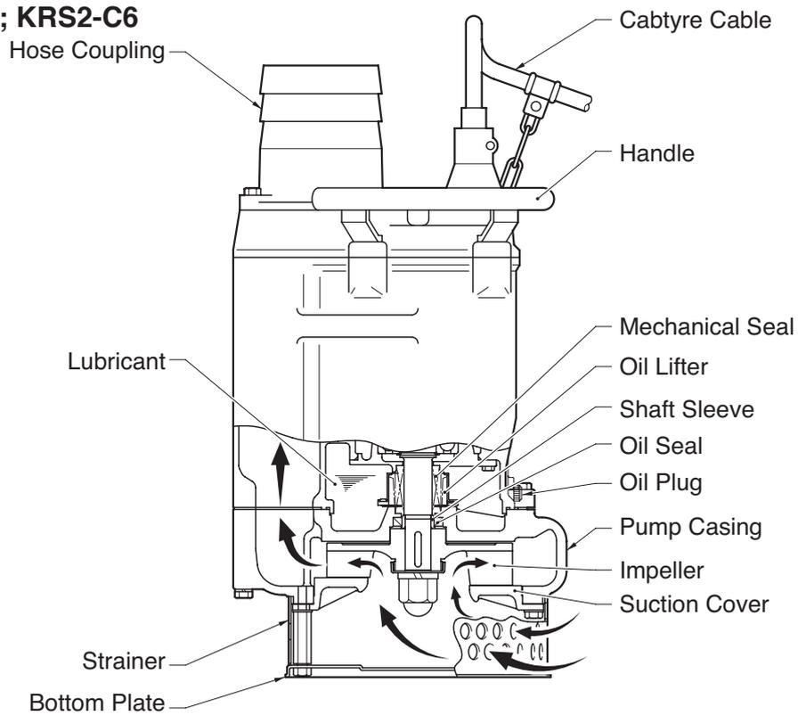
**Note:** *The above diagram is typical of the KRS2-C6, but some models may vary slightly in appearance or internal structure.*
