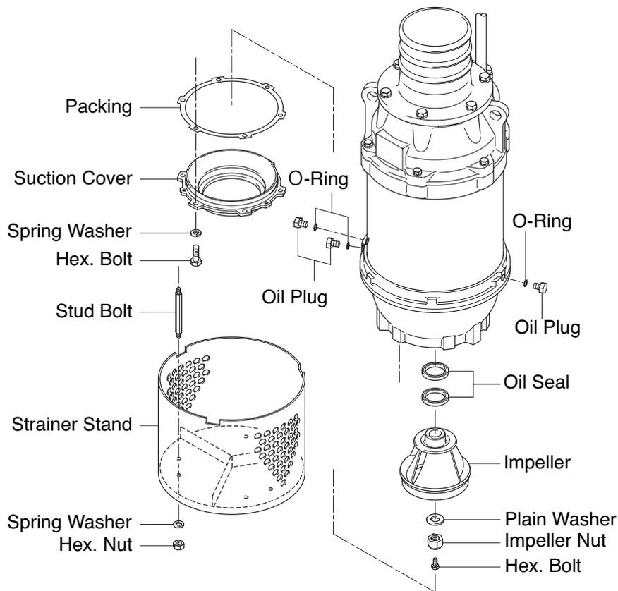
**Note:** The above exploded view is for model KRS1022. Other models may differ slightly in shape and construction.
